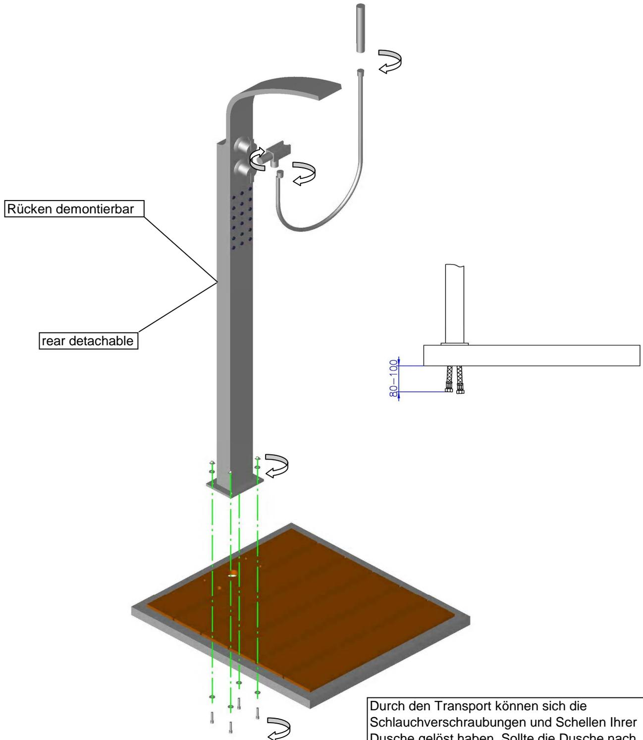
Transport may have loosened your shower's screw and bracket connections. If the shower leaks after first installation, please unscrew the rear and fasten the connections. Thank you.
